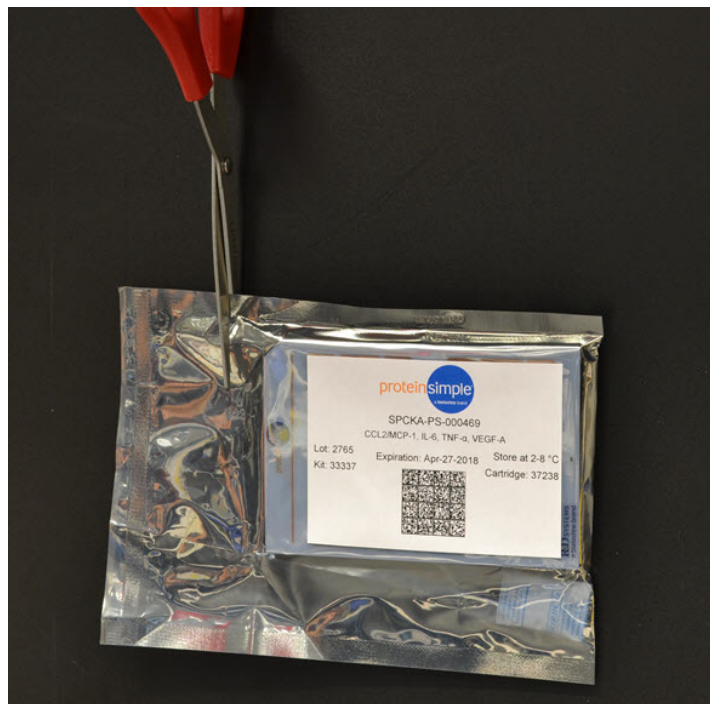
Figure 3-6: Removing cartridge protective casing.
