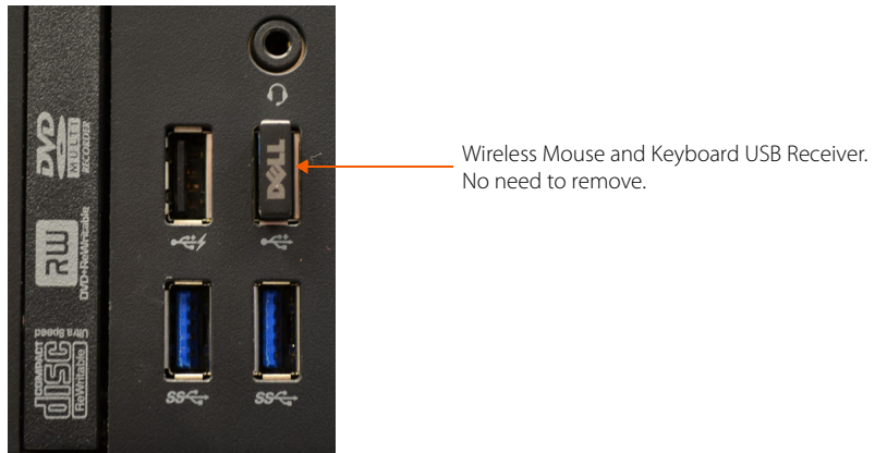
Figure 1-5: Front of PC close up of wireless mouse and keyboard receiver in USB Port.
